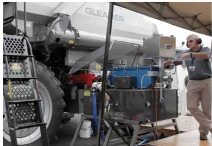
Customers enjoy this demonstration using a dynamometer to gauge the horsepower delivery at the main clutch shaft and show the torque curve characteristics on the new engine.
